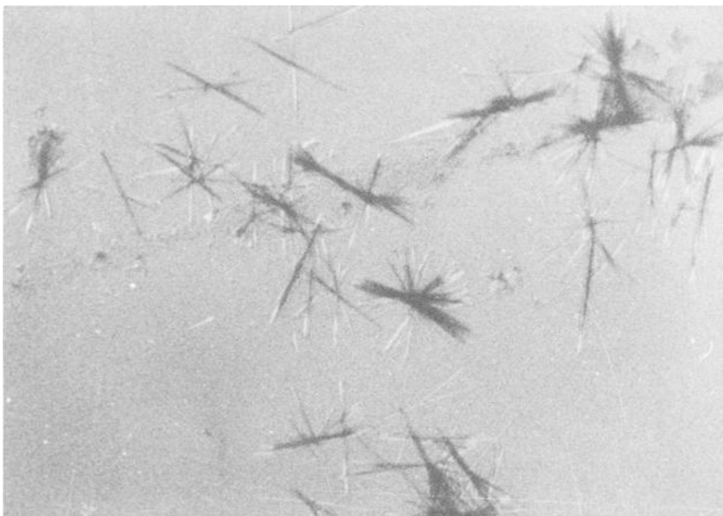
FIG. 1—Characteristic crystals of lead with dithizone.
